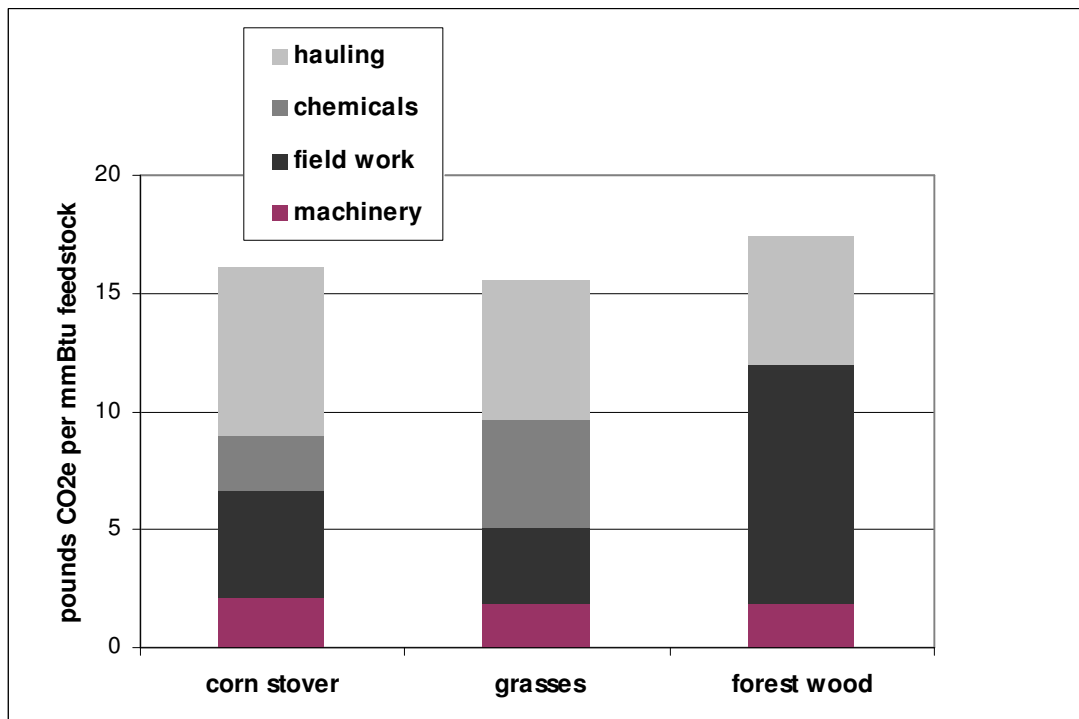
Figure 3: Total life-cycle CO 2 emissions from biomass feedstocks at each pre-plant production stage
